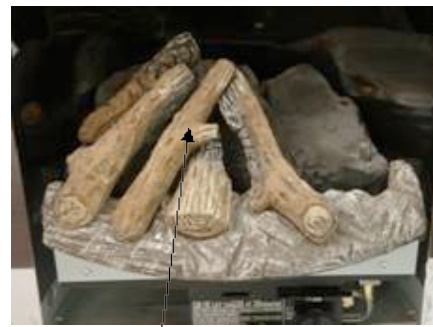
NEXT LOG SITS AS SHOWN INTO RECESS AT FRONT AND OVERLAPS LOG AT THE TOP
